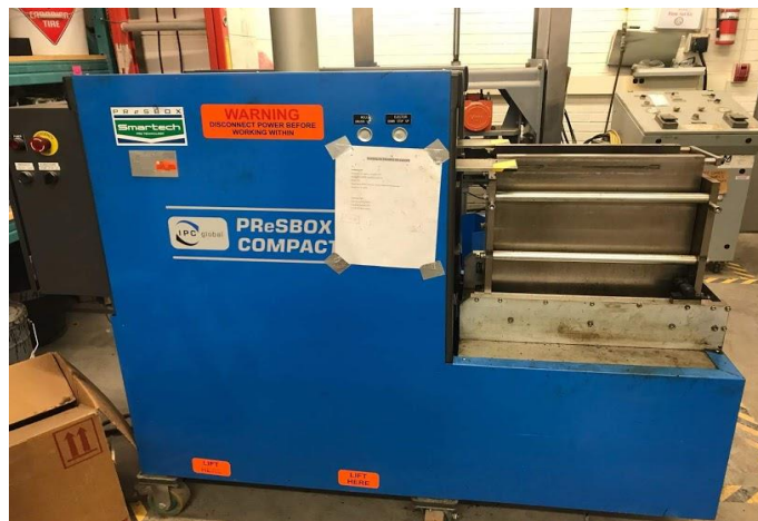
Figure 3-3 PReSBOX® Shear Compactor at the CPATT Lab, University of Waterloo
