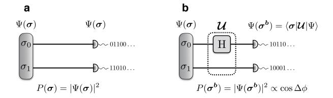
Figure 4.1: Unitary rotations for 2 qubits. a) Measurements on the reference basis. b) Measurement in the rotated basis. The unitary rotation (the Hadamard gate on qubit 0) is applied after state preparation and before the projective measurement.
