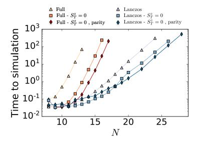
Figure 1.1: **Exact diagonalization**. We show the time (in seconds) required to reach the solution of the ED simulation for the 1d Heisenberg model. We carried out full diagonalization, where the whole spectrum is obtained, as well as the Lanczos algorithm targeting only the ground state. For both cases, we plot the results from considering the full matrix Hamiltonian, the  $S_T^z = 0$  sector and the parity/reflection symmetry. Simulation were performed using the library QuSpin [11].
