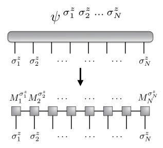
Figure 1.4: **Matrix product states**. Decomposition of a wavefunction into a MPS form, carried out via a series of singular values decomposition (not shown in the figure).
