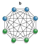
Figure 2.3: **Boltzmann machine**. **a)** Fully-visible Boltzmann machine. **b)** Boltzmann machine with hidden neurons (blue).
