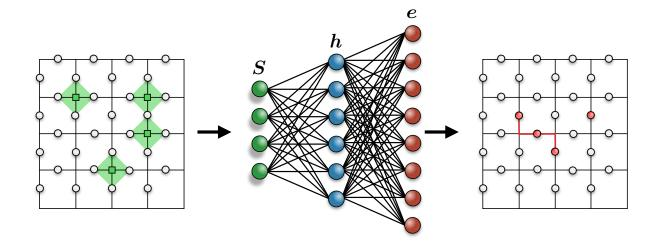
Figure 5.6: The neural decoder. The hidden layer h is fully-connected to the syndrome and error layers S and e After training, the syndrome is fed to the neural decoder, which generates a compatible error recovery chain.
