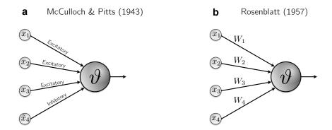
Figure 2.1: Early models of artificial neurons. a) The first model of artificial neuron, introduced by McCulloch and Pitts in 1943. b) The Rosenblatt perceptron neuron.
