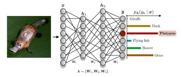
Figure 1.12: **Feedforward neural networks.** An image of a platypus is provided as input to a feedforward neural network. The pixel intensities are processed through the network and the output shows the probabilities for different animals (labels).
