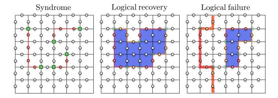
Figure 5.5: **Error correction**. a) An error chain e (red circles) and its syndrome S(e) (green squares). b) A successful recover chain (orange circles), creating a trivial cycle. c) A recovery chain generating a non-trivial cycle, and thus leading to a logical failure. This corresponds to apply the logical operators  $\hat{Z}_L^{(2)}$ .
