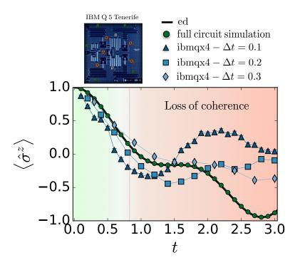
Figure 1.11: Quantum simulation with superconducting hardware. Quantum simulation of the time evolution of the TFIM for a quantum quench from h = 0 to h = 1. We compare the results from a simulation of the results from the ibmqx4 hardware, with results from ED (black) and classical circuit simulation (green).
