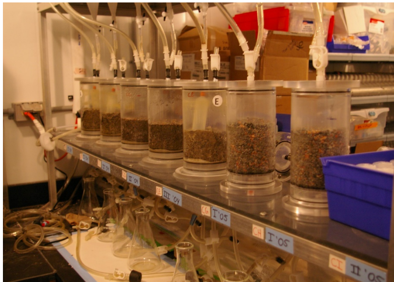
Figure 1.2 Cold temperature humidity cell experiment configuration.
