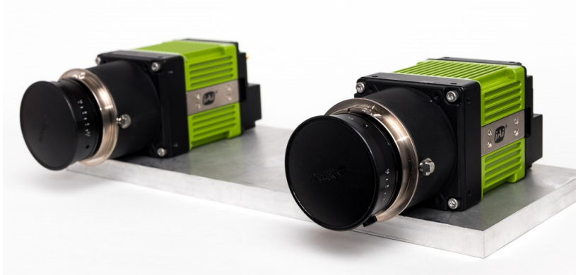
Figure 3.3: JAI SP-12000M high speed cameras with ZEISS 50mm f/2.2 lenses.
