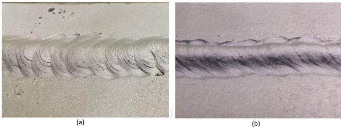
Figure 4-27: Bead appearance for welds performed at 45° downhill position by an experienced pipeline welder using (a) DC generator power supply, (b) Solid-state power supply.
