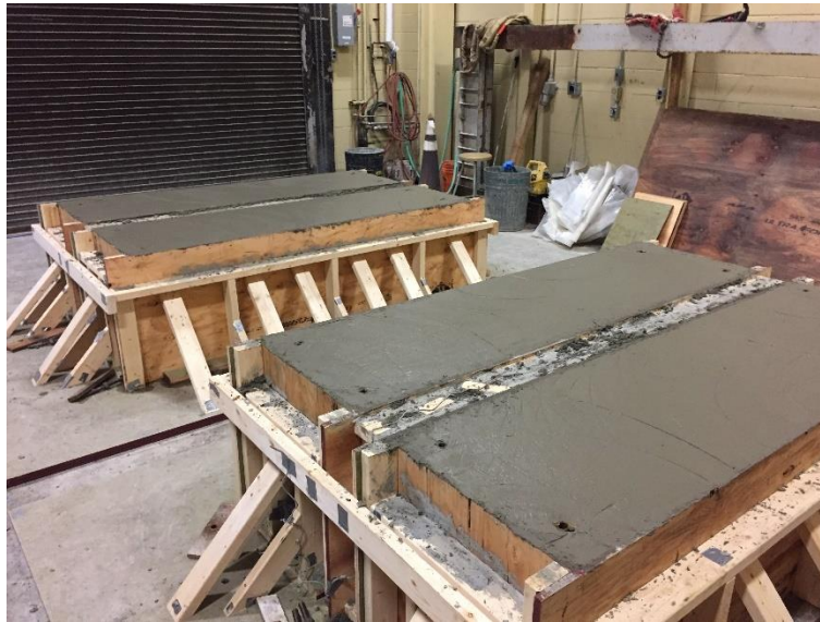
Figure 3.7: Picture of Fresh Concrete in Wooden Formwork for Beams B1
