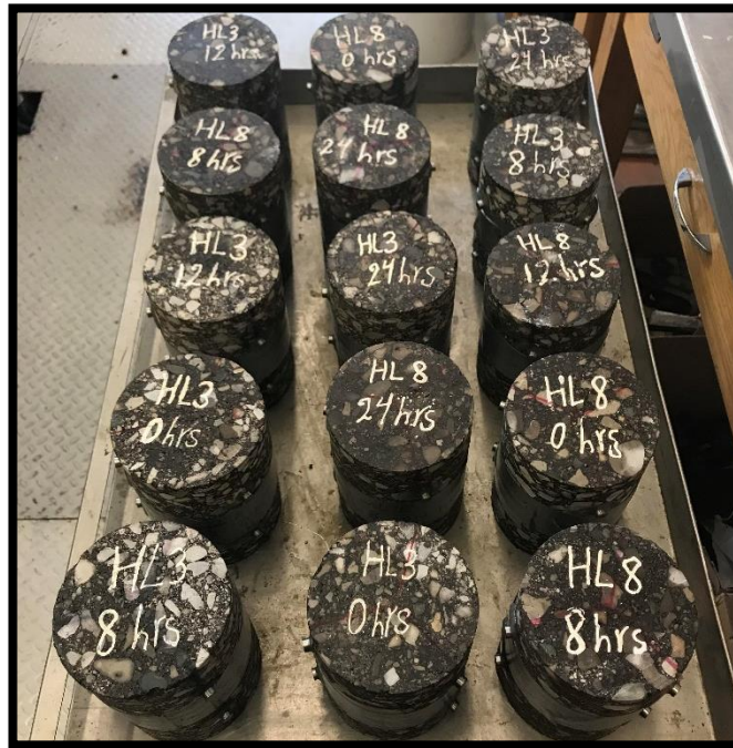
Figure 2: Dynamic modulus test samples after testing
