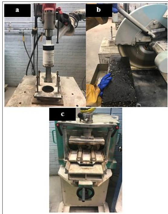
Figure 3-9 (a) coring machine, (b) saw-cutting machine, and (c) grinding machine
