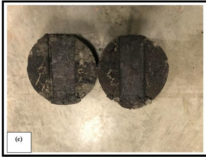
Figure 3: (a) Rutting samples under HWTD (b) & (c) rutting samples after testing
