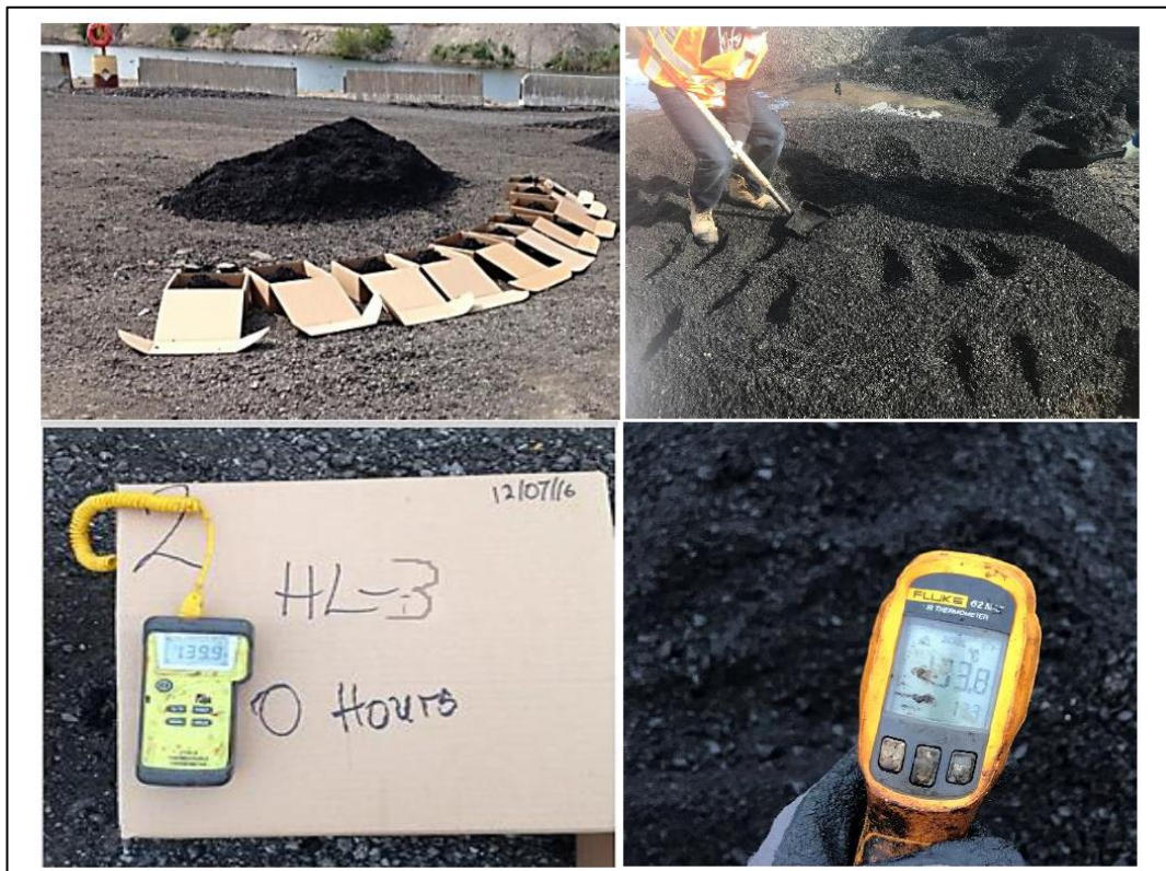
Figure 3-3 Monitoring the temperature of the collected mixes during sampling
