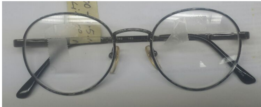
Figure 5.2. Patches of transparent Sellotape™ on the Plano glass to create disease models.
