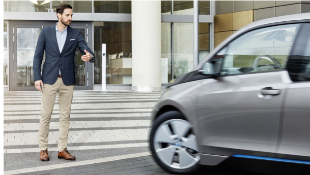
Figure 2.11: BMW i3 self-parking system: the vehicle recognizes gestures transmitted from an smart watch, and drives into and out of a parking space fully automatically. Image source: https://goo.gl/CyeKJd
