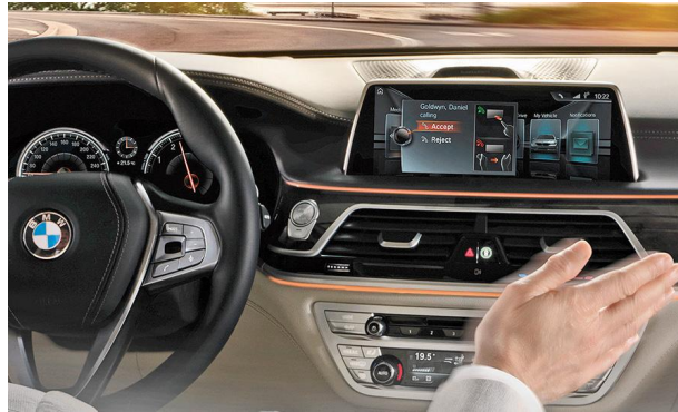
Figure 2.9: Car infotainment gesture control: SoftKinetic technology built in BMW car. The technology allows the driver to control the infotainment system with hand gestures.
