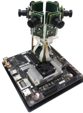
Figure 5.2: e-CAM30_HEXCUTX2 - Six synchronized full HD cameras for NVIDIA Jetson TX1/TX2
