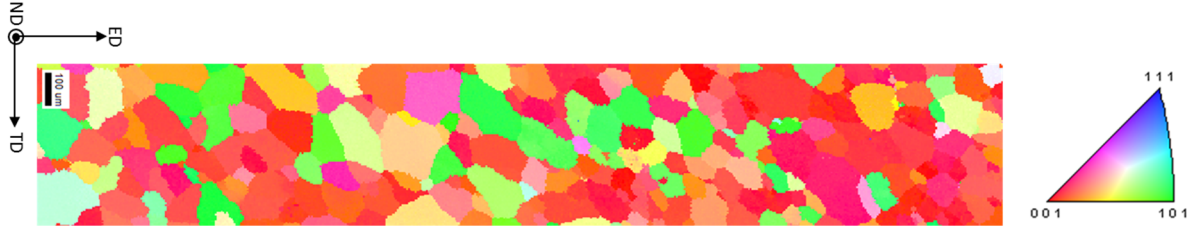
Figure 5-16: EBSD map of the input microstructure grain colors represent the crystallographic orientations.
