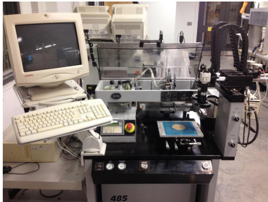
Fig 3.1: MSP-485 Screen Printer Machine in the CAPDS lab
