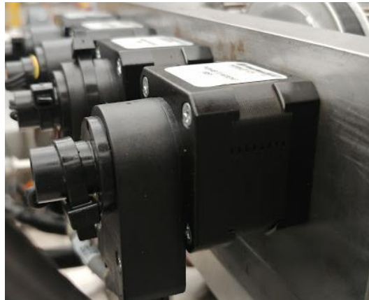
Figure 4.8: Linear actuators with encoders & home position switches
