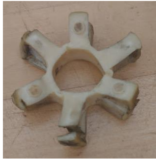
(a) Hytrel spider after testing
