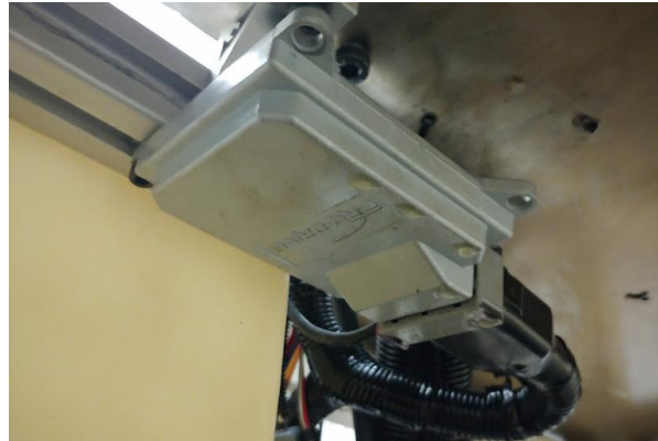
Figure 4.10: EFI ECU (mounted under table)
