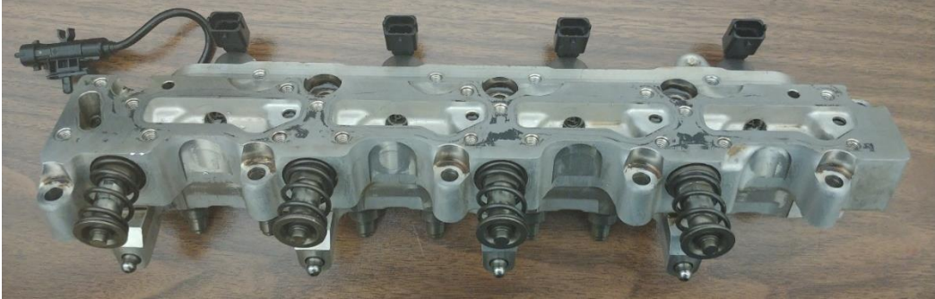
Figure 2.8: Disassembled Multiair unit
