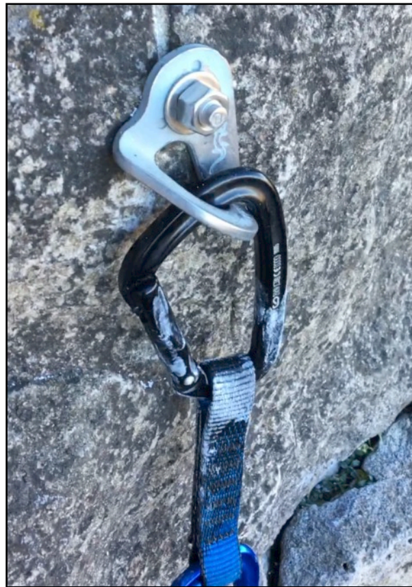
Figure 1. Bolt hanger with quickdraw attached. This is a screen-capture from my iPhone helmet camera.
