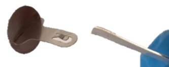
Figure 42: Gerstel clip (left) and the 0.2mm aluminum supported membrane (right)
