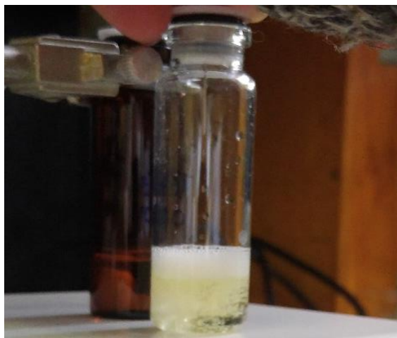
Figure 18: A foam layer on the oil upon vacuuming. The needle of the vacuum line can be seen in the top of the vial.
