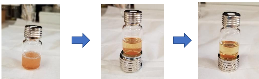
Figure 34: Image 1 shows the suspension of particles in cod oil after vortexing; this remained in suspension for 10 minutes as the particles extracted the analyte. Image 2 and 3 demonstrate the process for recollection of the particles to one location to facilitate collection with a blade.
