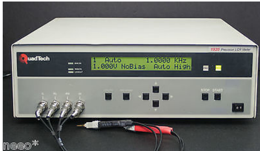
Figure A.5: LCR meter used in this study to measure gas hold-up in the recycle line
