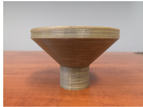
Figure 3.3: (a) Schematics of recycle cup design from U.S. patent No. 3124518 and (b) Fabricated recycle cup
