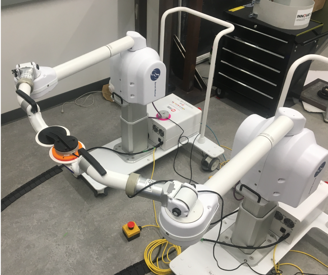
Figure 3.1: The experimental setup, two rigidly connected BURT manipulators in mirror configuration.
