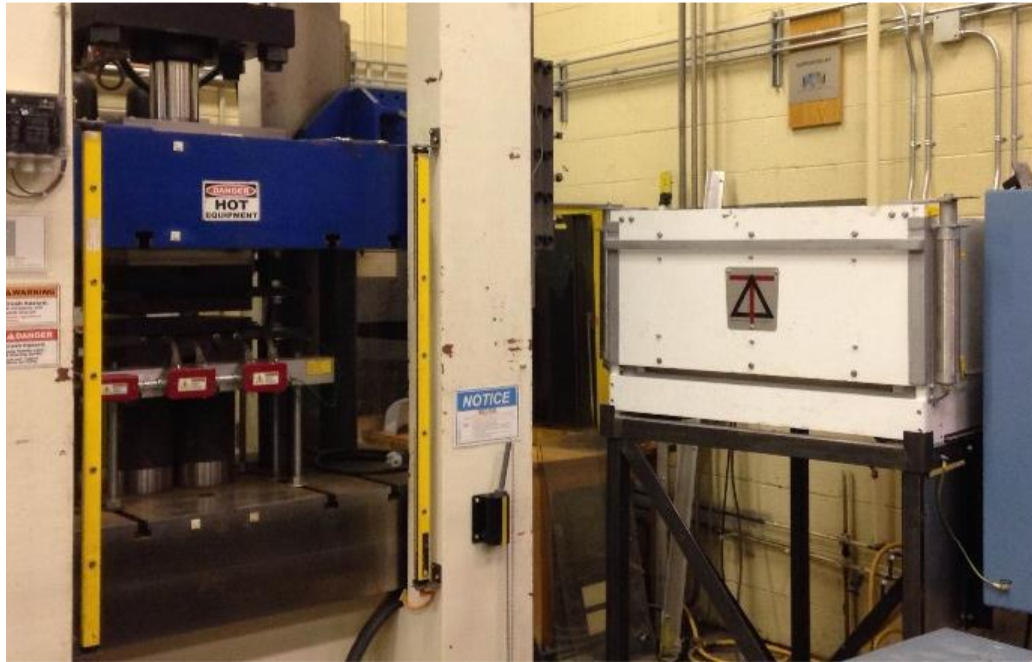
Figure 3.2 Macrodyne press with the automatic oven-transfer system used for the press-hardening operation
