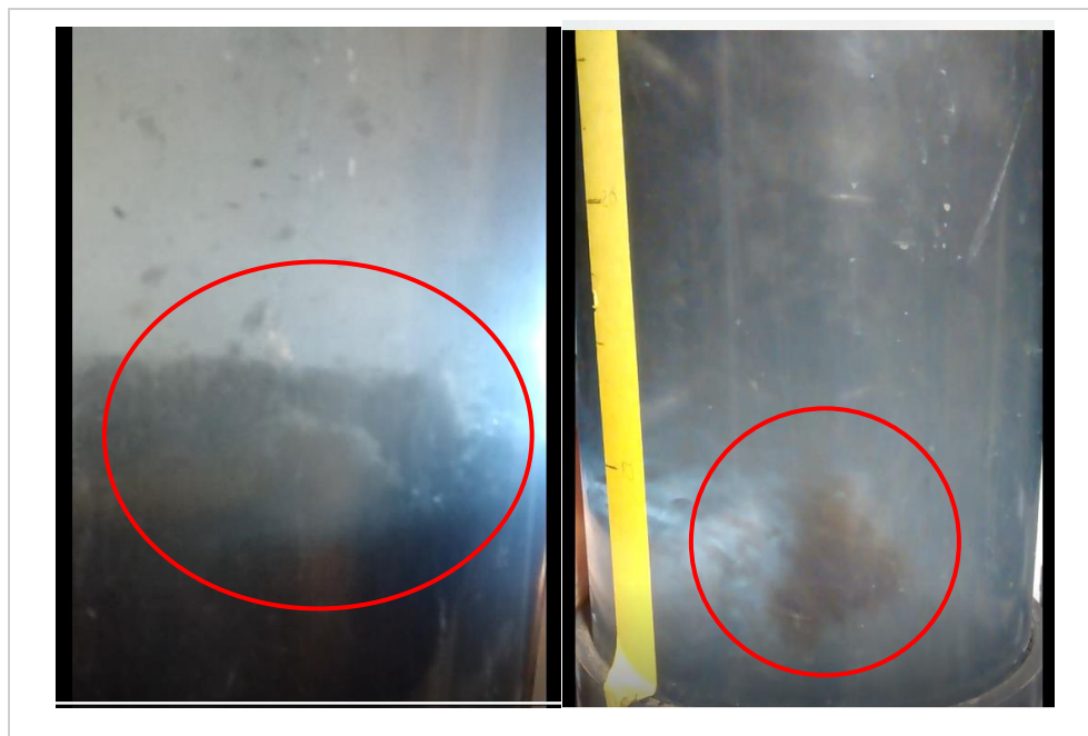
Figure 3.2: Solids masses emerging in Filter 4 (left) and Filter 2 (right) during backwashing on June 29 th , 2018.
