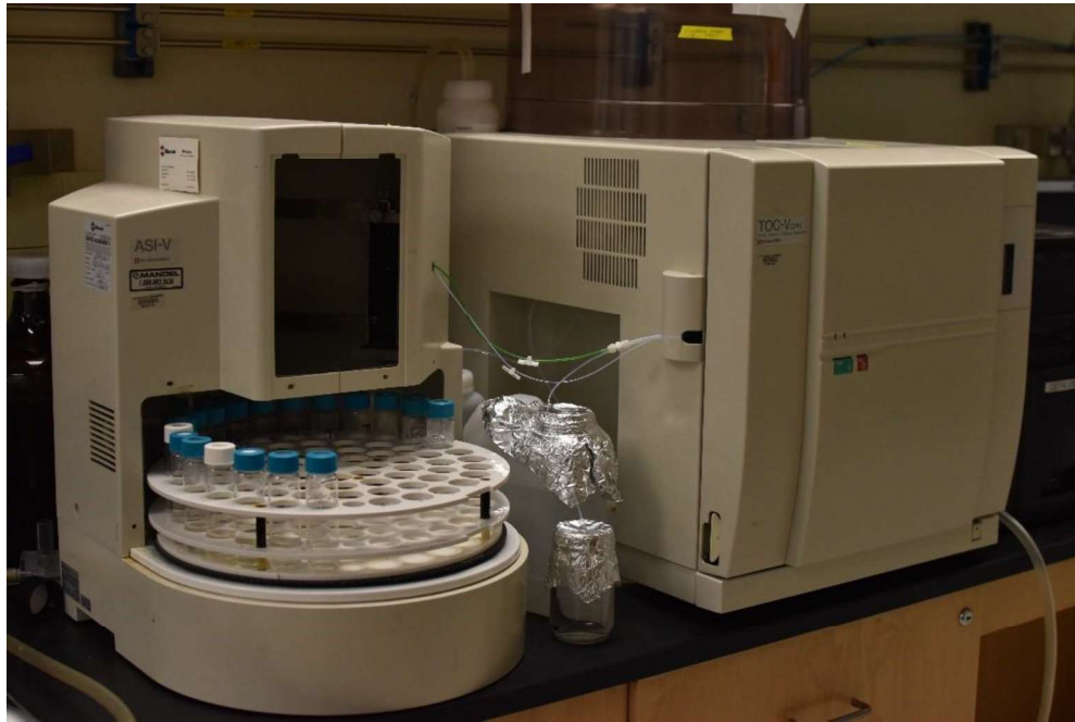
Figure 3-5 Shimadzu TOC-VCPH TOC analyzer used to measure DOC concentration.
