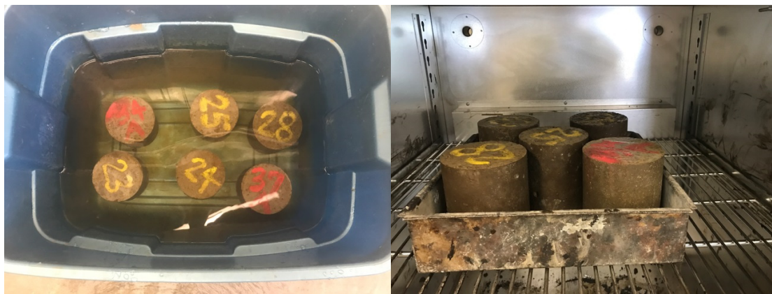
Figure 5-35 Testing of wetting and drying cycles. Soaking (left), and drying in oven (right)
