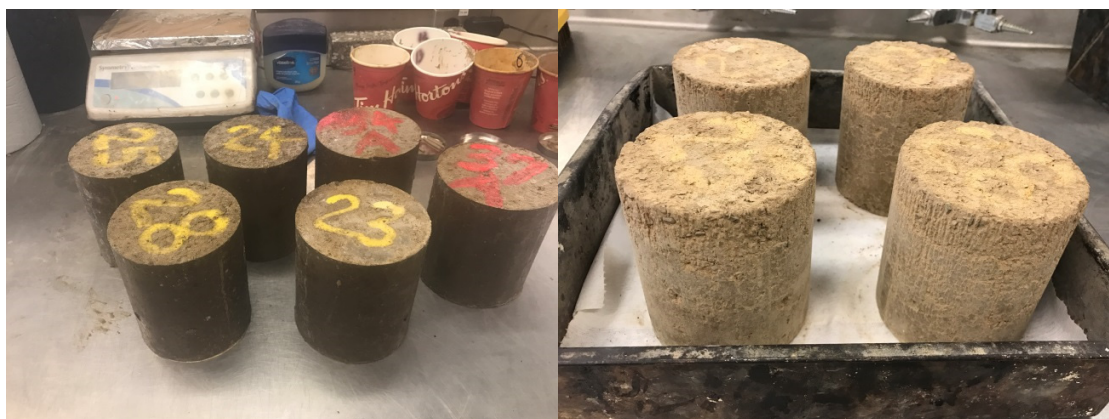
Figure 5-38 Dresden before cycles (left), specimens after 12 wetting and drying cycles
