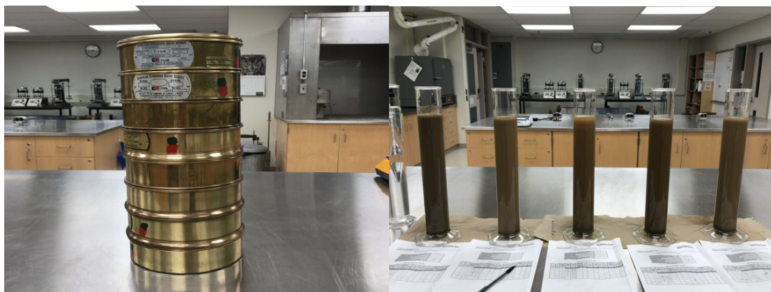
Figure 5-2 Sieves for sieving analysis (left), and sedimentation of hydrometer analysis (right)
