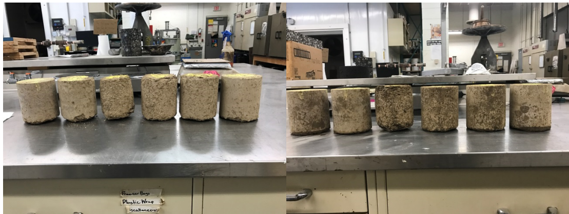
Figure 5-37 Blenheim after 12 freezing and thawing cycles
