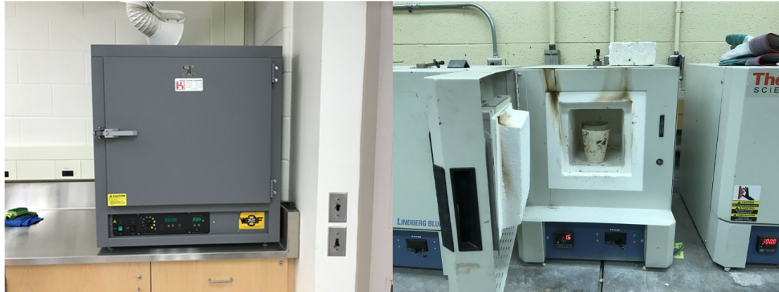
Figure 5-1 Oven for soil drying (left), furnace for organic matter ignition (right)
