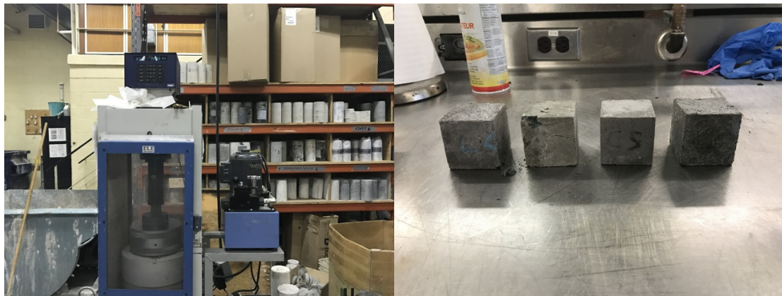
Figure 4-17 Testing of mortar cubes (left), cubes after testing (right)
