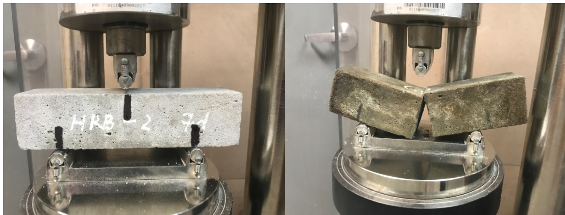
Figure 4-21 Testing of flexural strength (left), specimen after testing (right)
