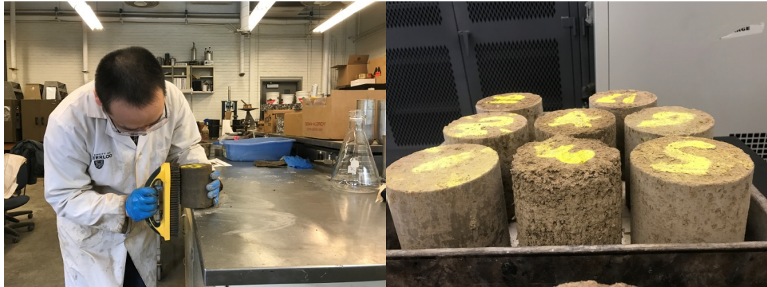
Figure 5-36 Brushing strokes at specimen's surface (left), specimens after brushing (right)
