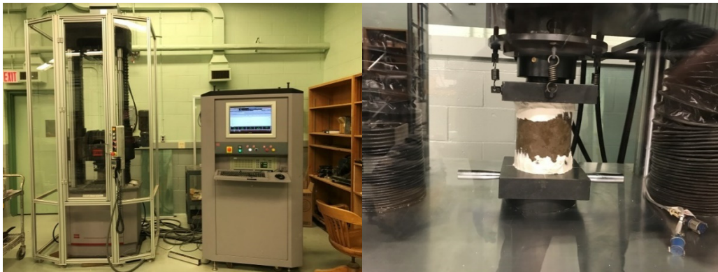
Figure 5-13 UCS test set up (left), UCS specimen during testing (right)
