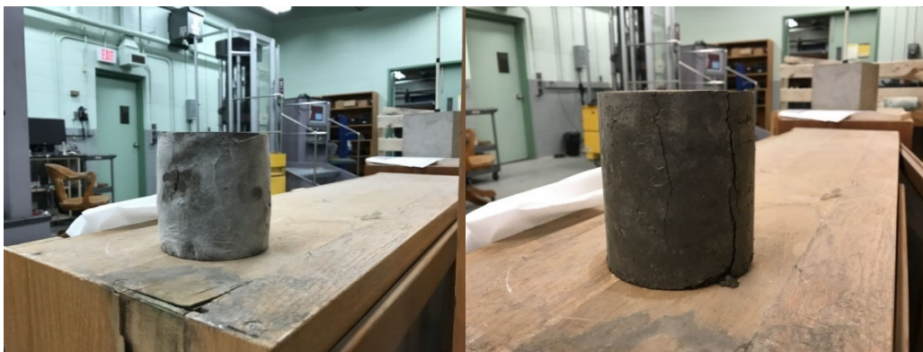
Figure 5-14 Specimens after testing: untreated Blenheim (left), treated Blenheim (right)
