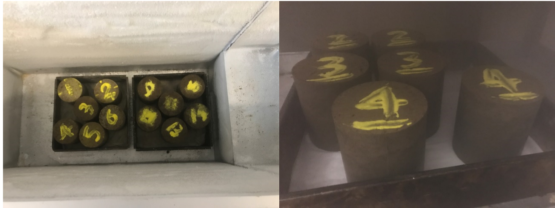
Figure 5-34 Testing of freezing and thawing cycles. Freezing in the fridge (left), and thawing in the humidity chamber (right)
