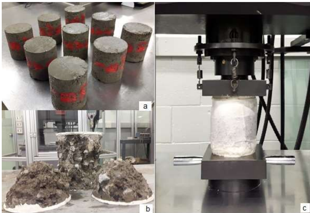
Figure 4.3 a) UCS specimens; b) shapes of UCS specimens after the test; c) UCS test on progress
