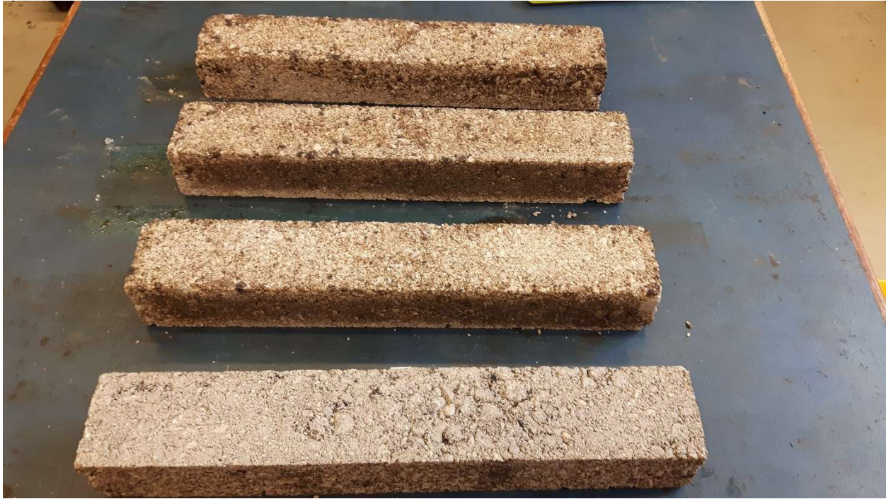
Figure 5.21 Condition of test specimens after fatigue test
