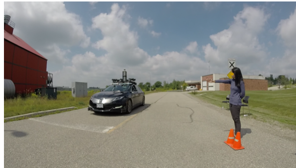
(c) Stop-and-Start Situation - Ego Stopped in front of the Crosswalk and Participant Indicating Decision to Cross with a Straight Arm Signal
