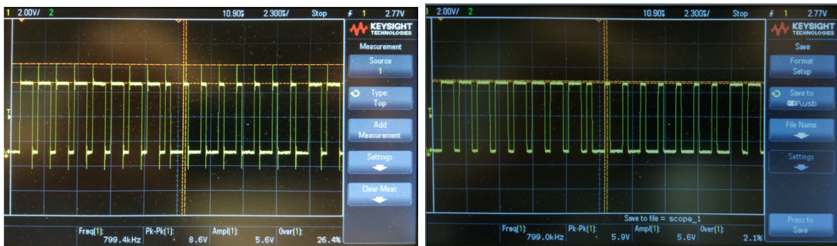
(a) Control Signal Before Impedance Matching (b) Control Signal After Impedance Matching
