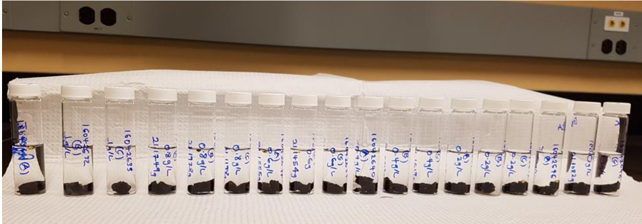
Figure 6-1: Vials containing Oil Sand + Starch Solution + Organic thinner before transfer into an Incubated Shaker
