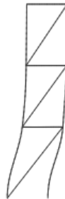
Figure 7.9: Buckled shape obtained from FEA of example one-bay, three-storey frame under proportional loading
