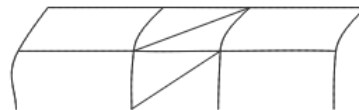
Figure 7.20: Buckled shape corresponding to the worst case fire scenario with single fire and floor separation constraints deactivated
