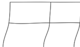
Figure A7.5: Buckled shape obtained from FEA of example two-bay, two-storey frame under proportional loading with considering shear deformations
