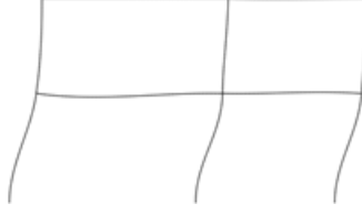
Figure 7.5: Buckled shape obtained from FEA of example two-bay, two-storey frame under proportional loading
