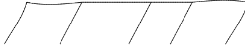
Figure 3.33: Buckled shape of modified four-bay frame in best case loading example obtained in ABAQUS (Simulia, 2012)
