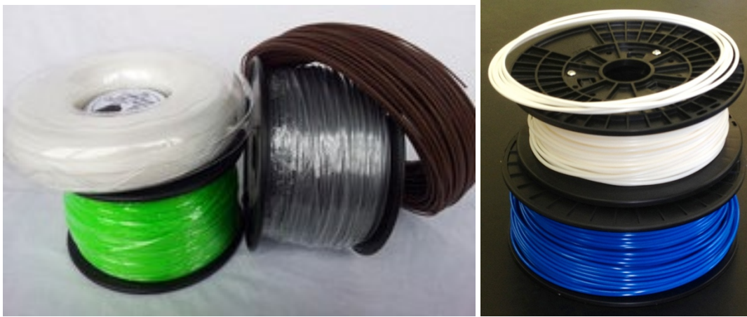
Figure 2.14 - 3.00 mm Thermoplastic filament spools typical of FDM processes.
