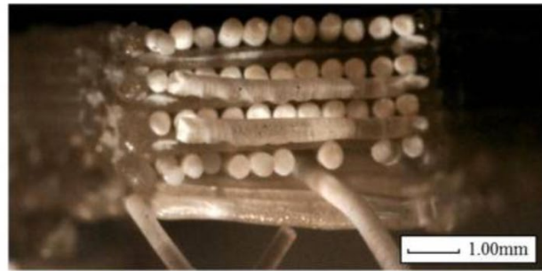
Figure 2.19 - i) diagram representing the typical hierarchical structure of an FDM assembled part and ii) microscope images of a fractured PLA FDM tensile specimen [92], [93]
