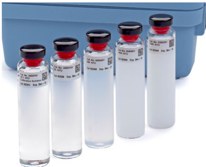
Figure 2.8 - Visible representation of turbidity in nephelometric turbidity units (NTUs) for <math><0.1</math>, 20, 200, 1000 and 4000 NTU [52]
