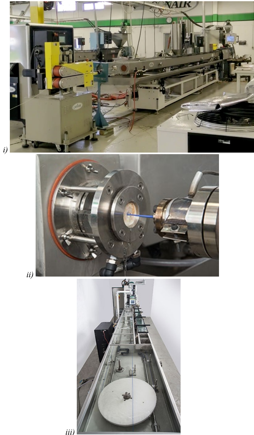
Figure 6.4 - i) commercial filament extruder at IPEG Conair North America equipped with a ii) Conair GRH-1.0 filament extrusion die and iii) HTMP multi-pass cooling and sizing tank [186]
