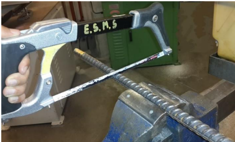
Figure 4.2. Creating rebar defects using a handsaw.
