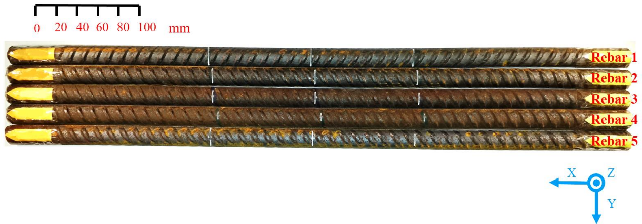
Figure 4.1. Prepared rebars with three symmetrically-located transverse cracks.
