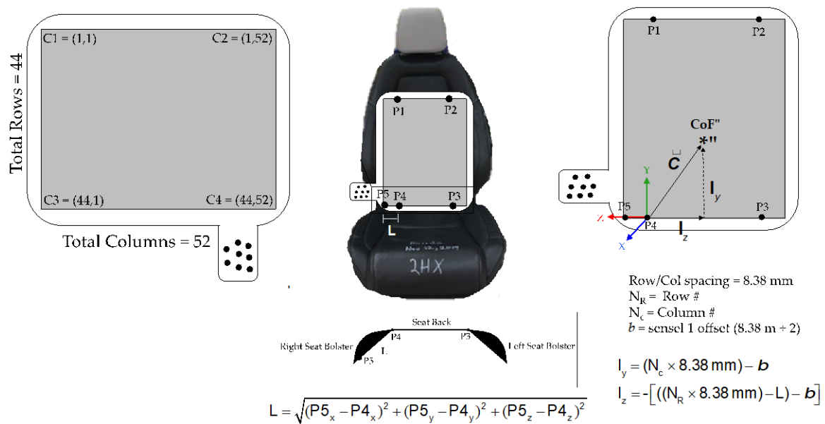
Figure 5.8: A schematic of the pressure mat setup. Left - the sensel number (X, Y) within the mat coordinate system are with respect to corner 1 (C1). Centre – the position of the pressure mat on the seatback and quantification of the row offset (L) and digitized points. Right - quantification of center-of-force coordinates with respect to the pressure mat local coordinate system.
