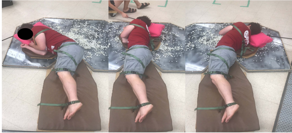
Figure 5.6: The frictionless jig positions. The figure displays the neutral position (center), which was used as the posture to secure the participant into the jig, extension trial (right) and flexion trial (left).
