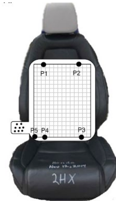
Figure 5.3: Location of the pressure mat with respect to the automotive seat and the 5 digitized points used to track the location of the pressure mat with respect to the seat and occupant.
