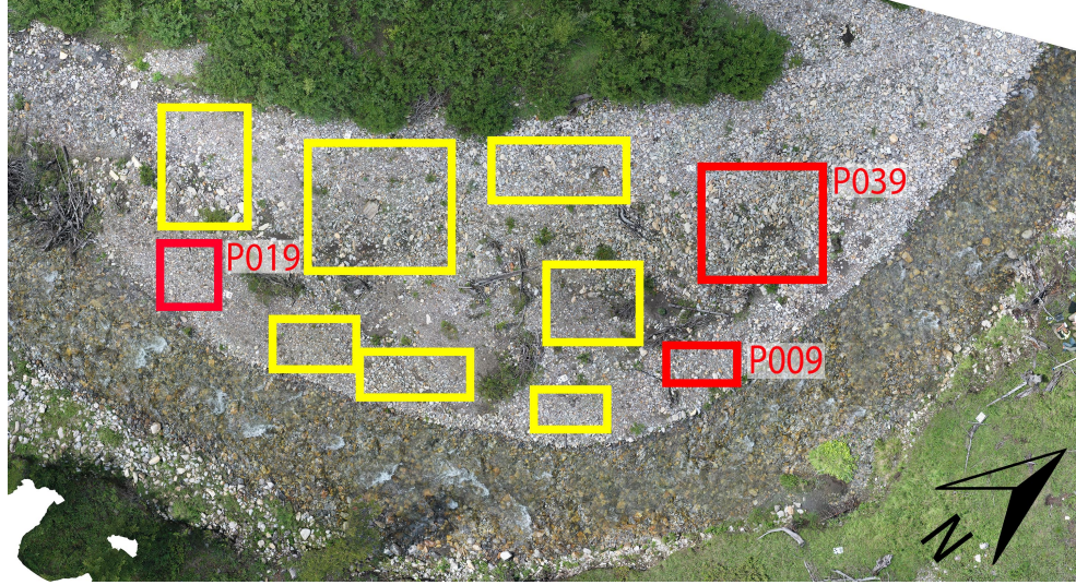
Figure 3-9: Example of BASEGRAIN measurement locations at a single survey location. Red rectangles indicate measurements that are shown in Figure 3-8 and yellow rectangles indicate additional measurements that were made along the point bar. The creek is flowing southwest.
