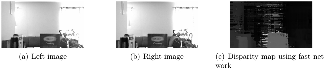
Figure 4.4: A rectified stereo image pair and its disparity map when the baseline is 47.8mm
