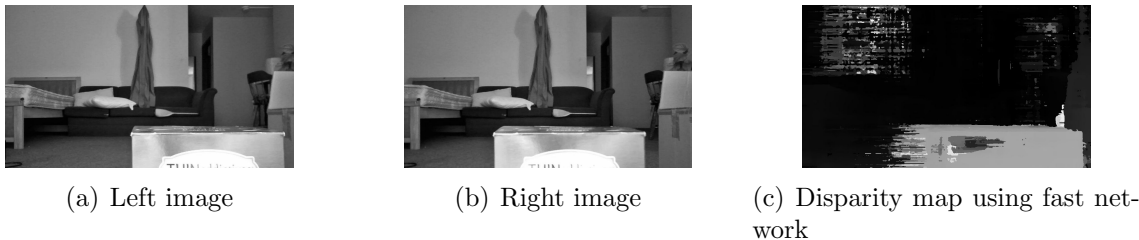
Figure 4.7: Example of a stereo image pair and its predicted disparity map affected by lens reflection
