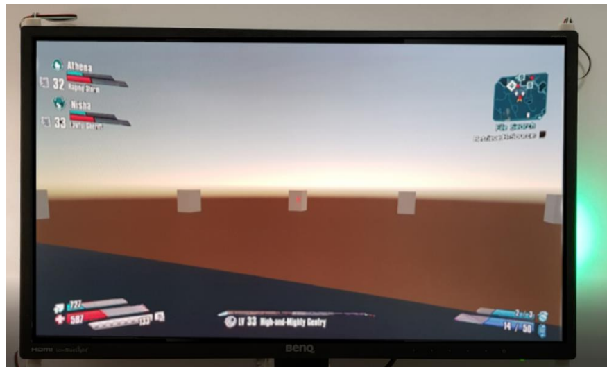
Figure 4.3: Ambient light indicator providing information on an objective to the right of the player.
