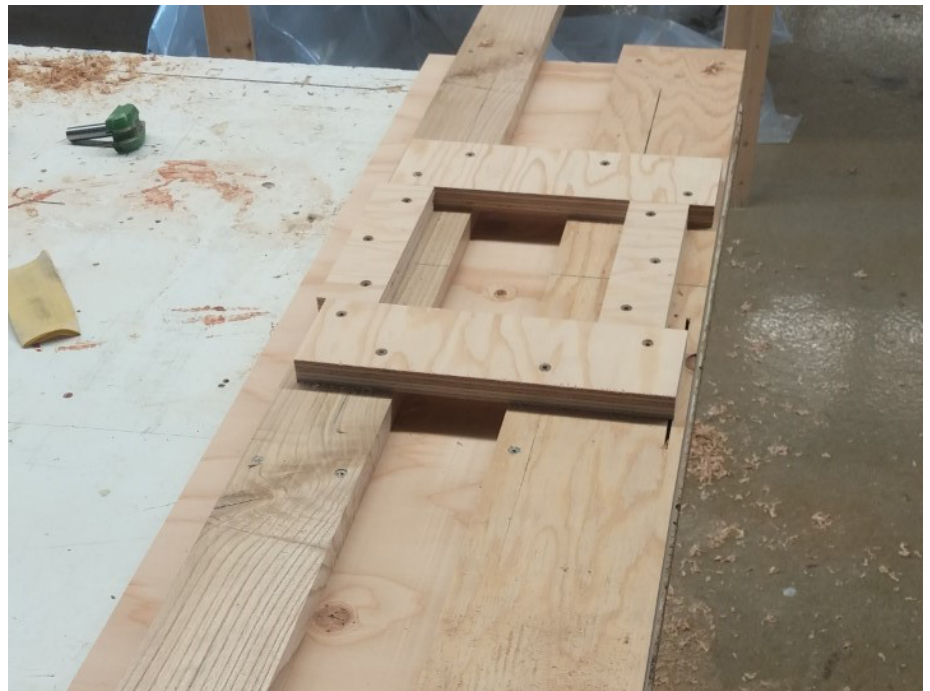
5.43 O Floor Lamp: Jigs made specifically for the projects to make the holes
