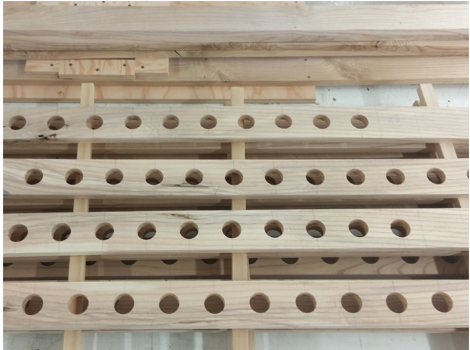
5.44 O Floor Lamp: First holes made with drill press
