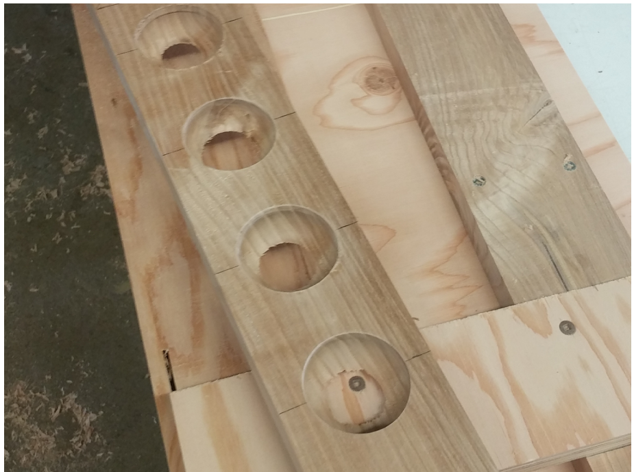
5.45 O Floor Lamp: Second holes made with router and jigs
