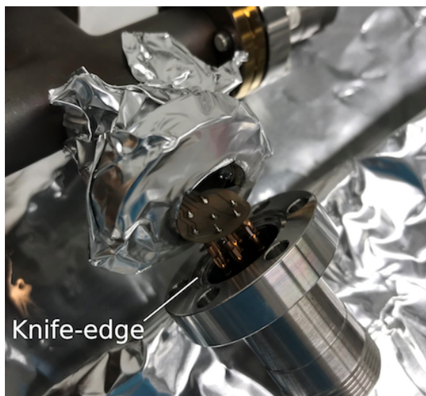
Figure 6.1: Example of a CF flange on a previous project.
