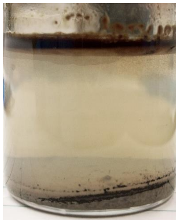
Figure E1. A picture of the extraction mixture using fresh oil sands ores and 1 g/L of Cat0.036-HB1.9-SNP after phase separation for 16 h at rt. At the bottom, the layer of black sediment on top of sands was very noticeable.
