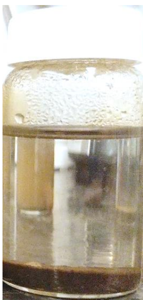
Figure E3. A picture of the extraction mixture using the aged oil sands ores and 0.25 g/L of Cat0.17-PHE0.38-SNP after phase separation for 16 h at rt. The supernatant was mostly free of suspended particles and emulsified bitumen droplets.
