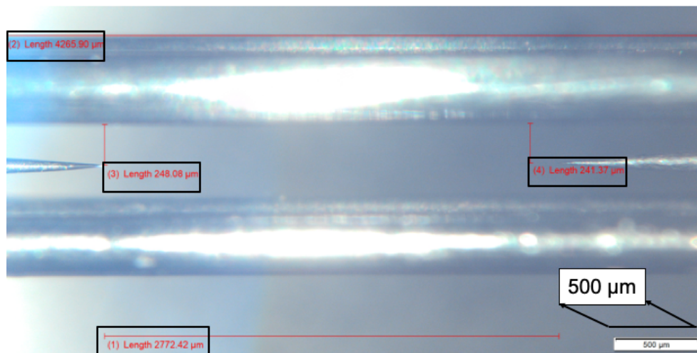
Figure 2.12: The exact alignment and geometrical parameters of the six-electrodes as used in our ion trapping apparatus
