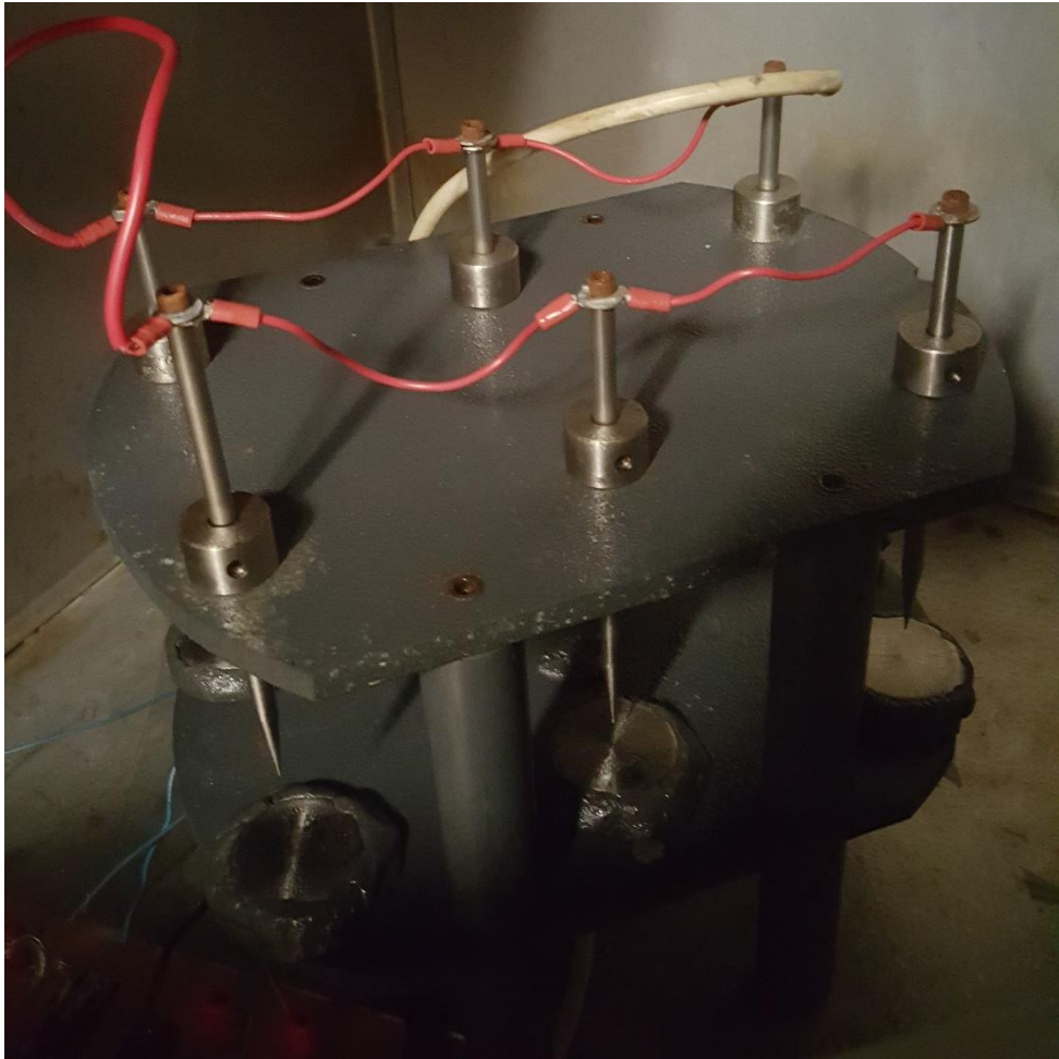
Figure 3.2. The structure of six pairs of electrodes used in generating corona discharges.
