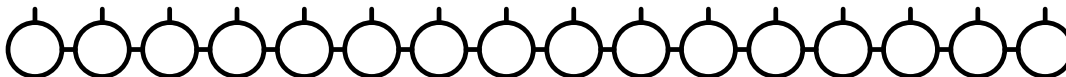
Figure 1.4: Pictorial representation of a matrix product state decomposition of a rank-16 tensor into rank-2 and rank-3 tensors. The vertical line segments correspond to the site indices. The contraction performed by the horizontal line segments may be interpreted as matrix multiplication.
