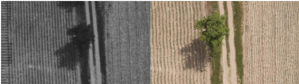
Figure 18: (Left) Image acquired with the multispectral sensor on the Parrot Sequoia that did not experience the rolling shutter effect, (Right) Image acquired with the RGB sensor on the Parrot Sequoia that experienced the rolling shutter effect.
