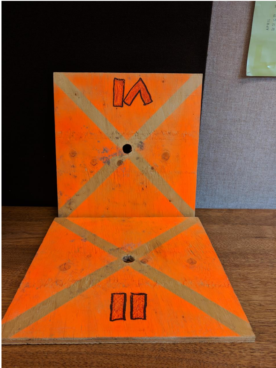
Figure B: Example of GCP used during the RPAS imagery acquisition.
