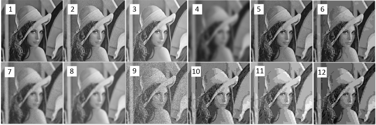
Figure 6.8: Out-of-sample images with different types of distortions having MSE = 500 : (1) stretching contrast, (2) Gaussian noise, (3) luminance enhancement, (4) Gaussian blurring, (5) impulse noise, (6) JPEG distortion, (7) Gaussian blurring + Gaussian noise, (8) Gaussian blurring + luminance enhancement, (9) impulse noise + luminance enhancement, (10) JPEG distortion + Gaussian noise, (11) JPEG distortion + luminance enhancement, and (12) JPEG distortion + stretching contrast.
