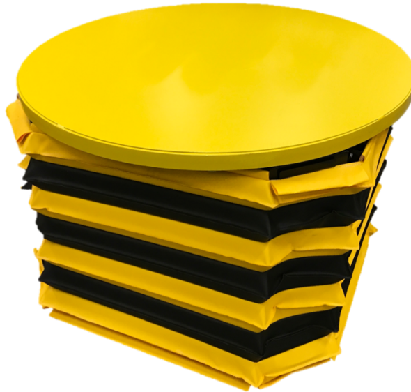
Figure 7-2: Self-leveling pallet utilized in the experiment (Southworth, Portland, USA)
