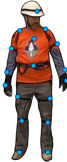
Figure 3-4: Photo of a mason wearing Axis Neuron (Noitom Ltd, 2017) motion capture. IMU locations are marked with blue dots
