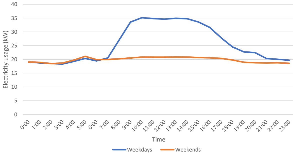
Figure 14 The hourly profile of aggregated electricity usage for plug loads of Tenant A, Tenant B, Tenant C, and Tenant D on weekdays and weekends, January – December 2019
