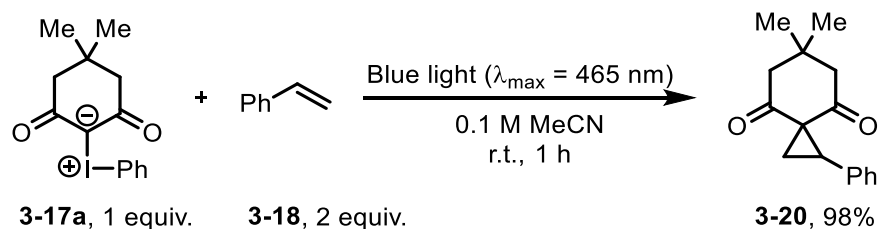
Scheme 3.7. Cyclopropanation reaction of iodonium ylides and alkenes under blue light.
