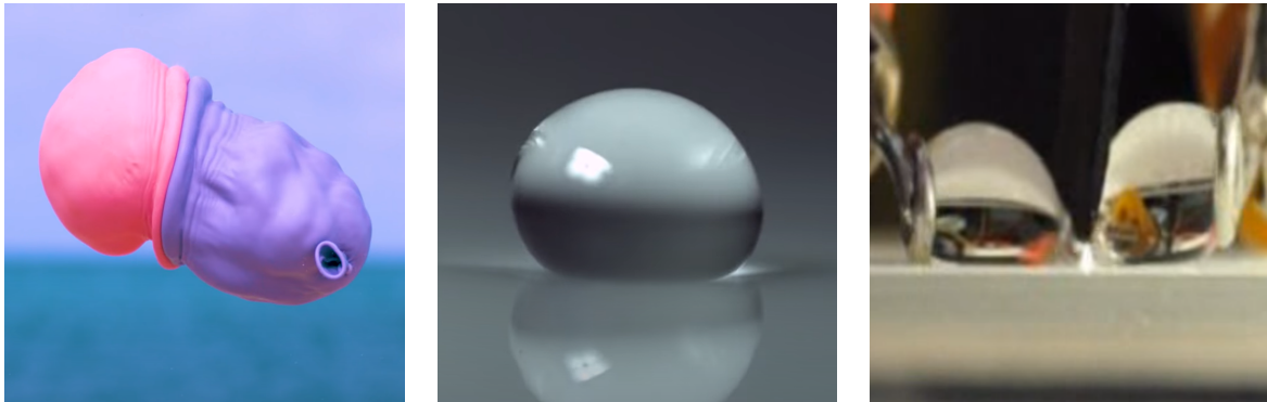
(a) Two water-filled balloons collide. (b) A droplet lands on a water surface and bounces off. (c) A droplet is cut by a hydrophobic knife.
