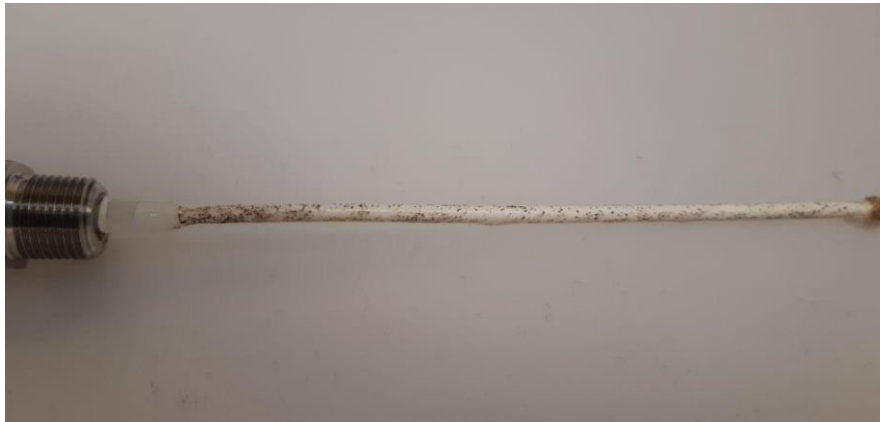
Figure B-8. Porous needle of a solution sampler clogged by CoFe-NPs (black areas) (SP-1 and SP-2) during the CoFe-NP transport and binding experiment. For the binding experiment, it was found that the CoFe-NPs had a physical interaction with the samplers (SP-1 and SP-2), which caused complete clogging of the porous needle. No interactions were observed between the porous needle in the Fe-NPs transport experiment. Linley (2019) reported that the only difference between the CoFe-NPs (lower coating concentration) and the Fe-NPs (higher coating concentration) is a larger morphology of CoFe-NPs (Figure B-1). Since most of the CoFe-NPs were retained in the crude-oil zone, and less NP mass passed below this zone, aqueous samples were able to be collected from the samplers located below the crude oil zone; however, the representativeness of these samples of the pore water concentration is uncertain.
