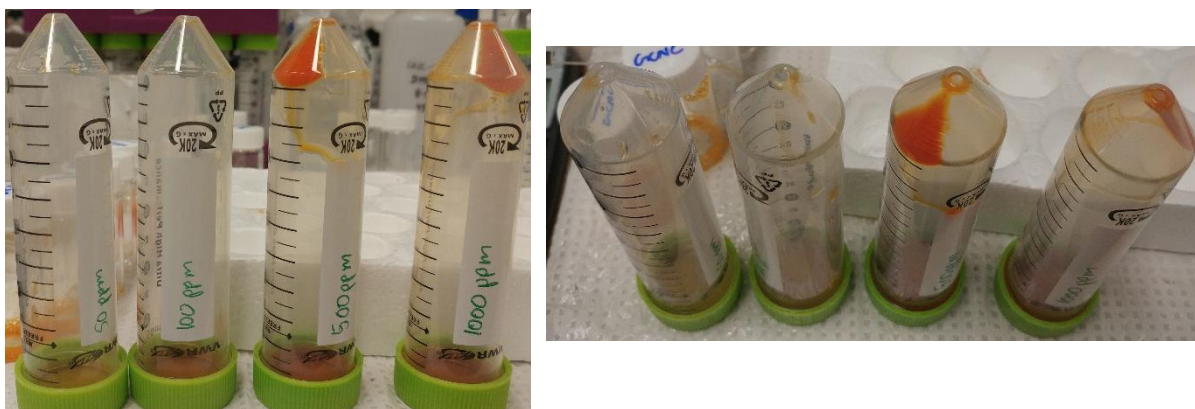
Figure 23: Pellets obtained after centrifugation of MO samples with GCNC as the adsorbent.
