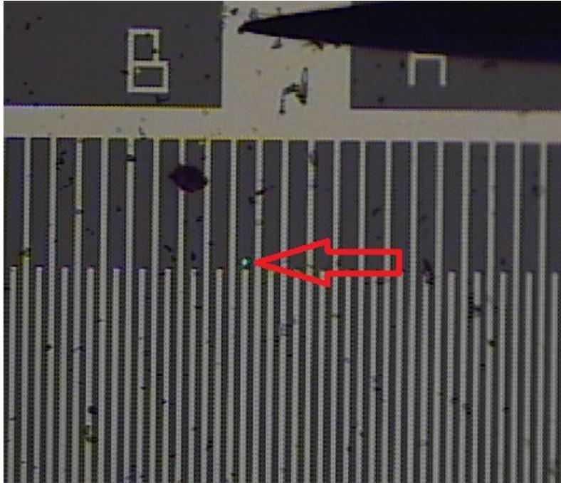
Figure 5.27: A microscopic image of the fabricated IDT for the BG wave resonator, showing the location of the Laser Doppler Vibrometry (LDV) laser spot.
