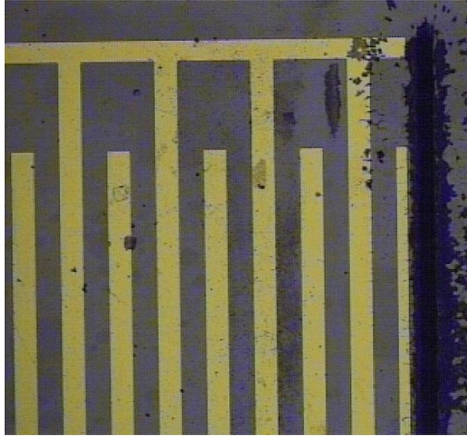
Figure 5.17: Localized heat damage near the trench due to the laser trimmer.
