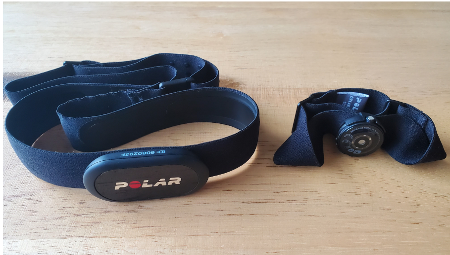
Figure 3.1: Polar heart rate monitors. (left) Polar H10, a chest strap device capable of transmitting ECG, HR, RRI, and accelerometer data over Bluetooth. (right) Polar OH1, an armband optical device capable of transmitting PPG, HR, PPI, and accelerometer data also over Bluetooth.
