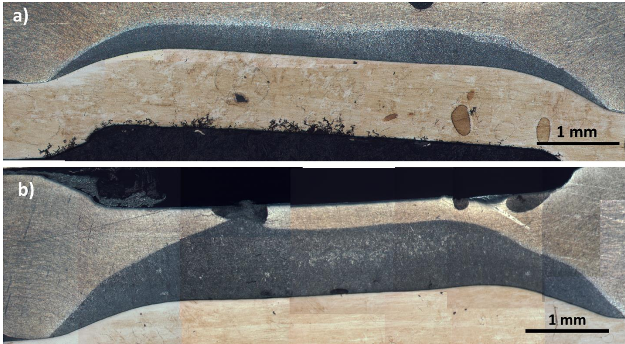
Figure 66 Microstructure of AZ81A coated sample at (a) 13 kA, (b) 14 kA without shielding gas
