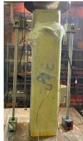
iv) Final Damage
