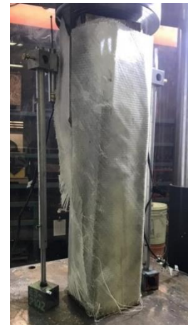
iv) Final Damage
