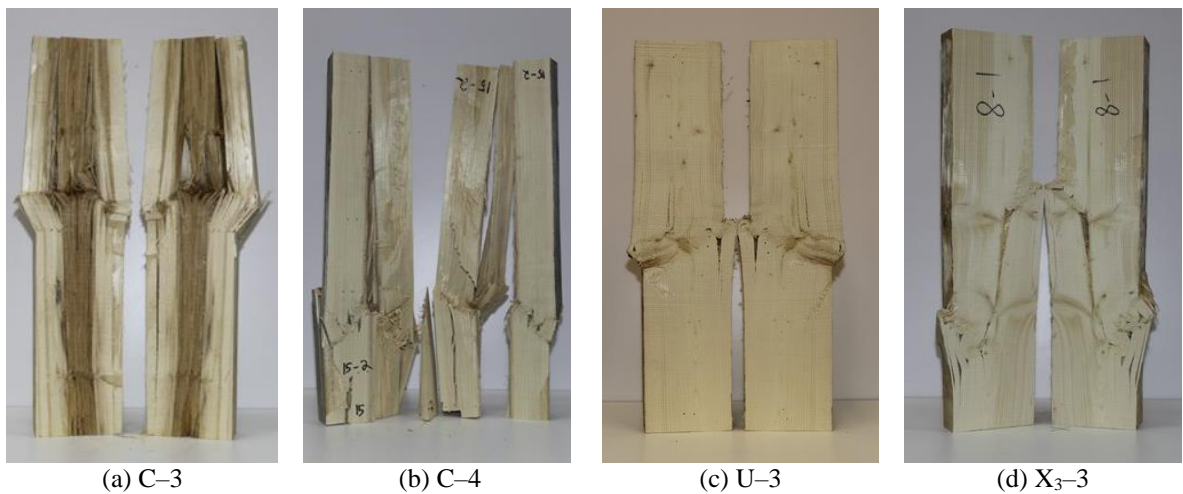
Figure 5.5: Final Damage States of Control Specimens vs. Reinforced Specimens
