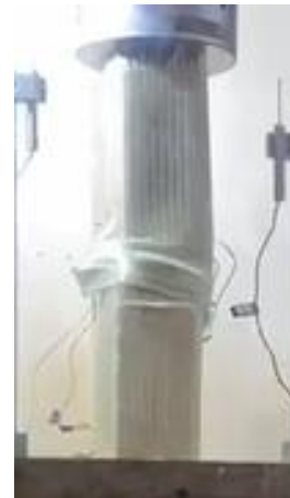
iv) Final Damage at 0.065 mm/mm
