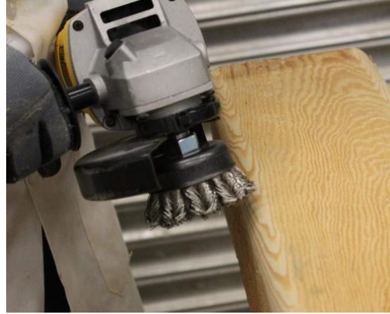
(b) Wire Brushing Rounded Corner to Roughen
