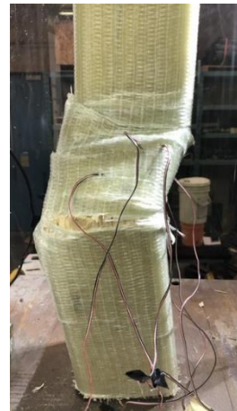
iv) Final Damage at 0.13 mm/mm strain
