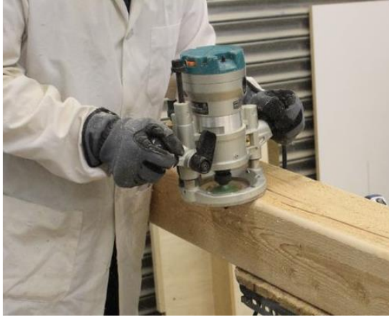
(a) Rounding Cross-Section Corner with Router
