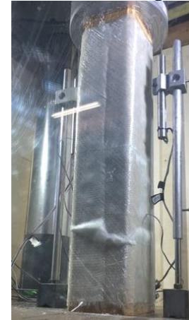
ii) Failure Initiation
