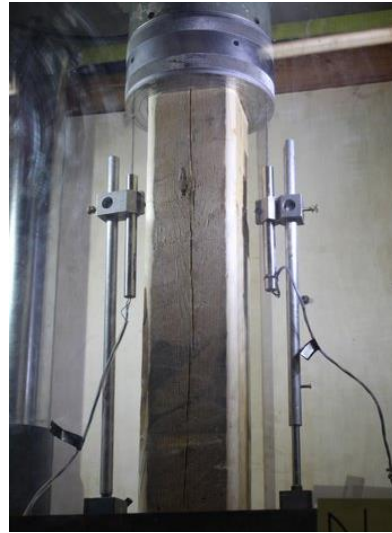
(b) Specimen and LVDTs setup for test
