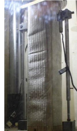
ii) Wood Rupture, Fibre Wrinkling
