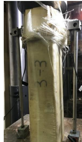
iv) Final Damage
