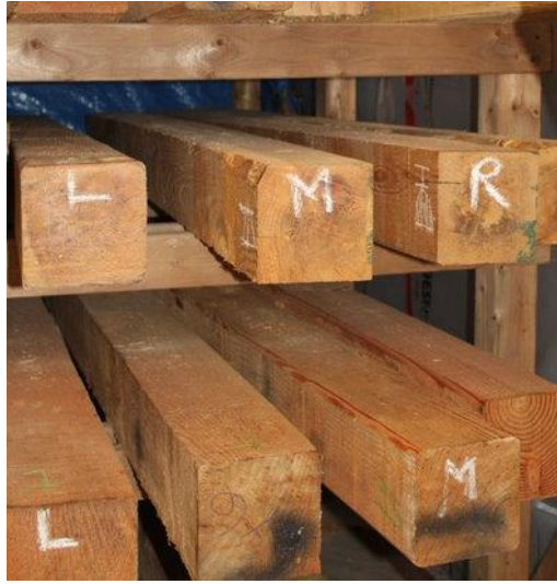
Figure 3.1: Storage of Material Lengths as Delivered
