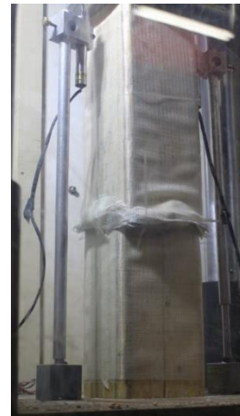
iv) Final Damage
