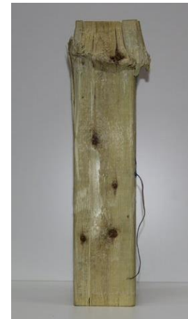
v) FRP Removed
