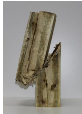
vi) FRP Removed 0.25 mm/mm Strain Damage
