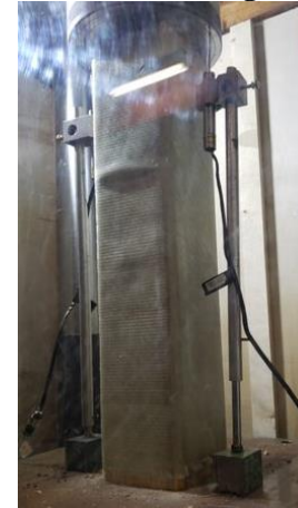
ii) Crushing Plane
