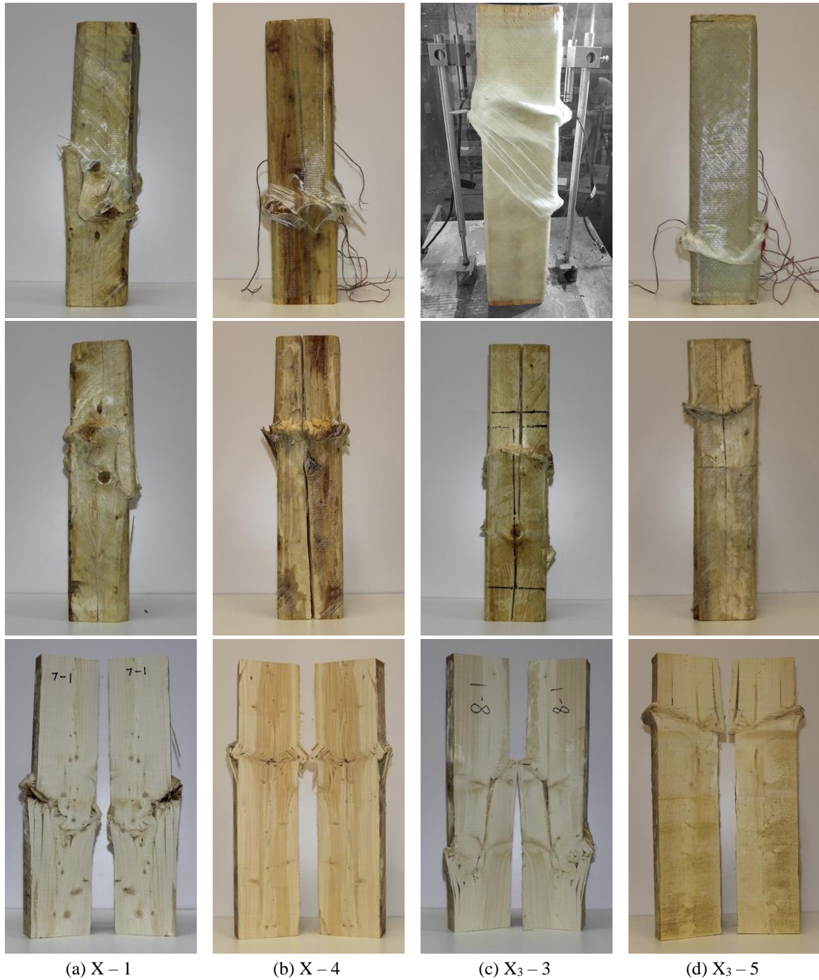
Figure 4.6: X & X 3 Representative Specimens Post-Test, FRP Removed, Dissected
