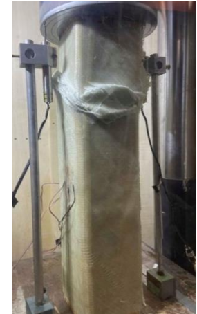
iii) Failure Propagates
