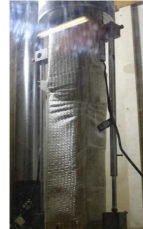
iii) Propagation, Fibre Rupture
