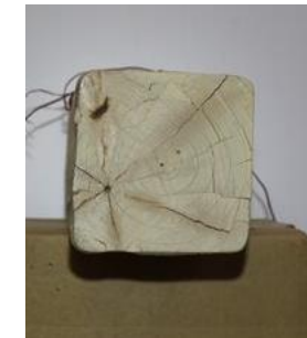
v) End Grain Damage
