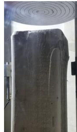
iv) Final Damage
