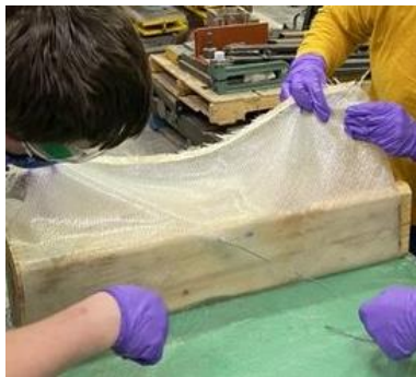
(c) Wrapping Fabric Over Prepared Specimen
