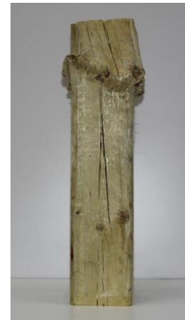
v) FRP Removed
