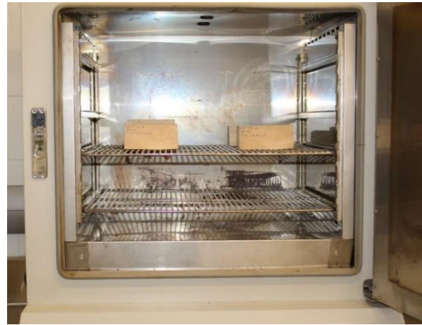
(b) Typical Sample Arrangement in Oven
