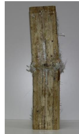
v) FRP Removed
