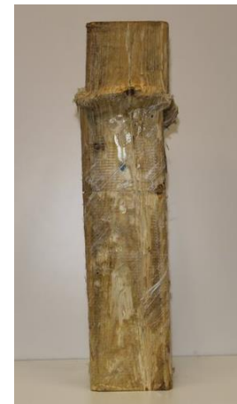
v) FRP Removed
