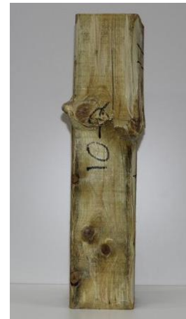
v) FRP Removed
