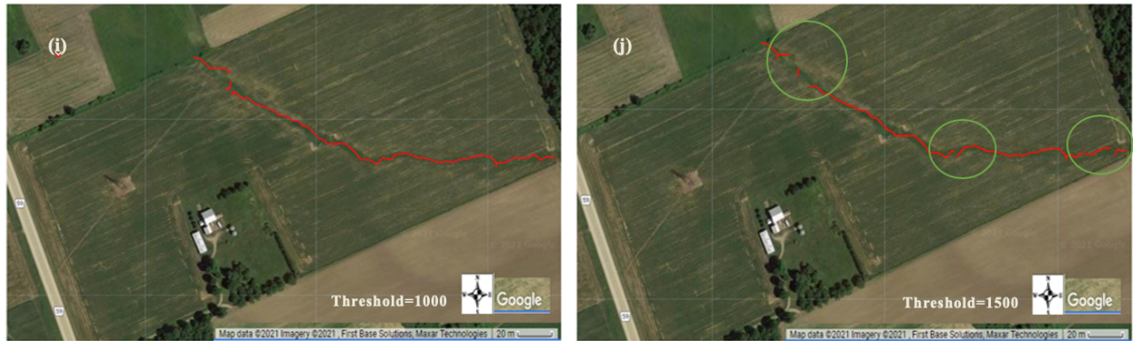
Figure 4.2.1. The Procedure of threshold finding. The predicted GWs are denoted by red lines. The significant discontinuities are denoted by green circle.
