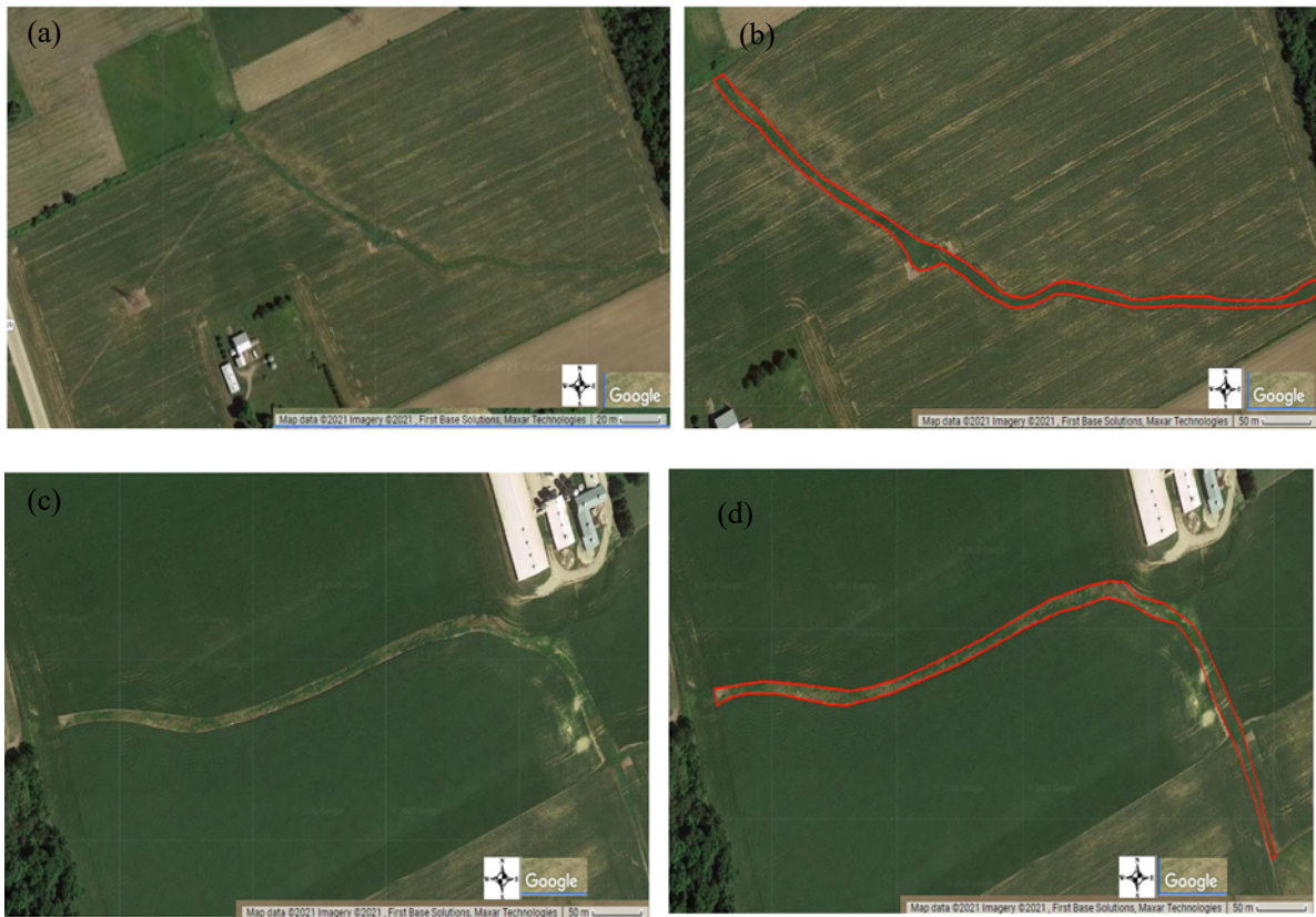
Figure 4.1.1 Example of digitized GWWs. (a) identified GWW (near 80^{\circ}48'52.165''W , 43^{\circ}14'55.992''N ). (b) close view of digitized GWW of (a). (c) identified longest GWW ( 80^{\circ}58'55.285''W , 43^{\circ}11'53.147''N ). (d) close view of digitized GWW of (c)
