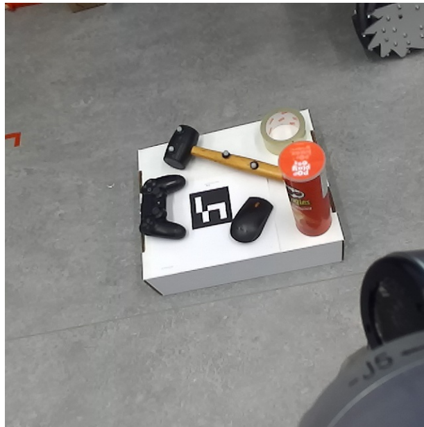
Figure 3.7: Mallet Object with Vicon Markers
