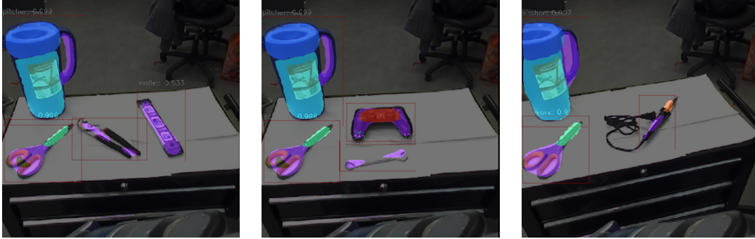
Figure 5.5: Affordance Detection of Novel Objects. The colour of the mask represents the affordance label. Grasp: purple; screw: orange; cut: teal; wrap-grasp: light blue; contain: dark blue; clamp: red.
